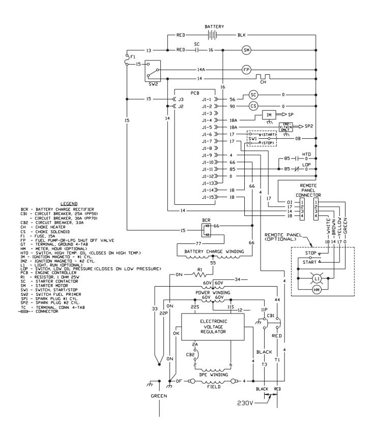
PRIMEPACT 50 and 70 (50Hz) Recreational Vehicle Generators Wiring Diagram & Electrical Schematic - Drawing No. 0D6579
